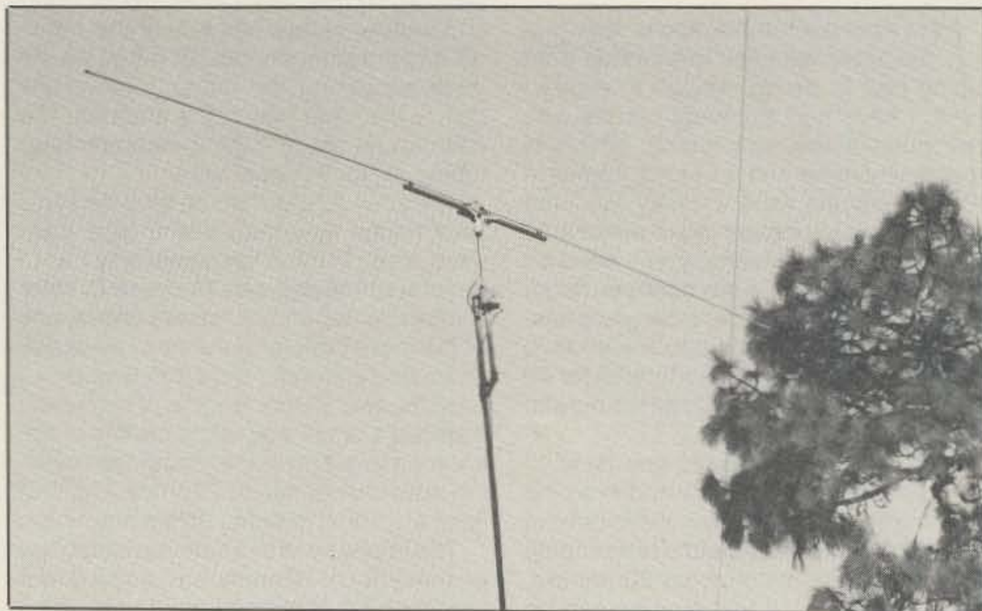
Here is another view of K4TTO's antenna. He employed a U100 lightweight rotor to turn the antenna. He also used Penetrox on all connections.
